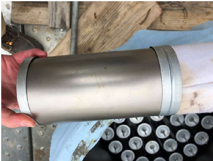
Figure 2. Blank Top Section of the element.
