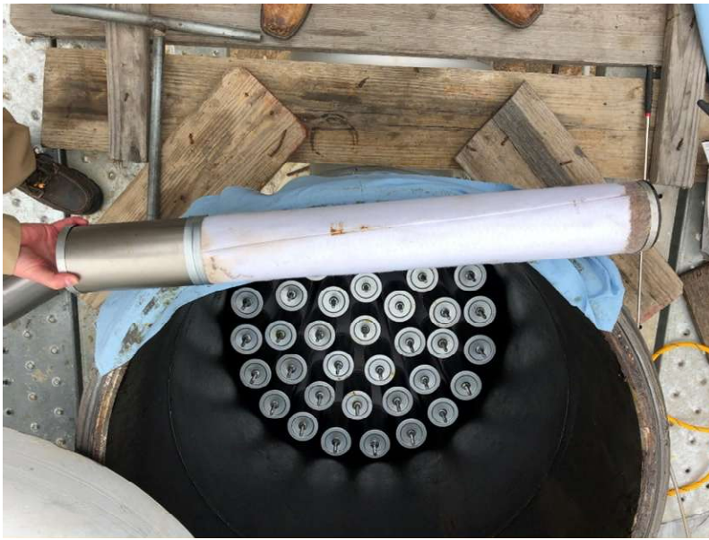
Figure 6. Spent Element, showing a Brown Band of Oil Seepage at the Bottom
